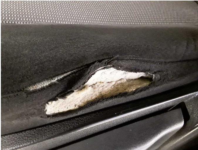
Damage 7: Seat - front: Seat upholstery - left side (inkl. Bezug) - Broken / torn - Replace
