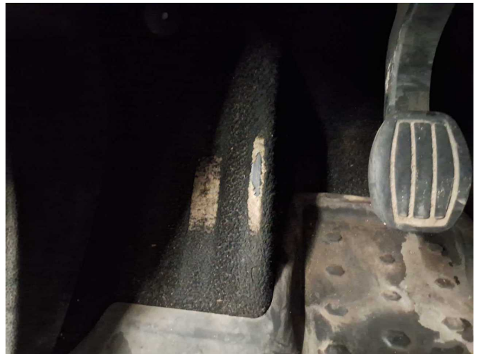
Damage 10: Trim / covers: Carpet - front left side - Broken / torn - Replace
