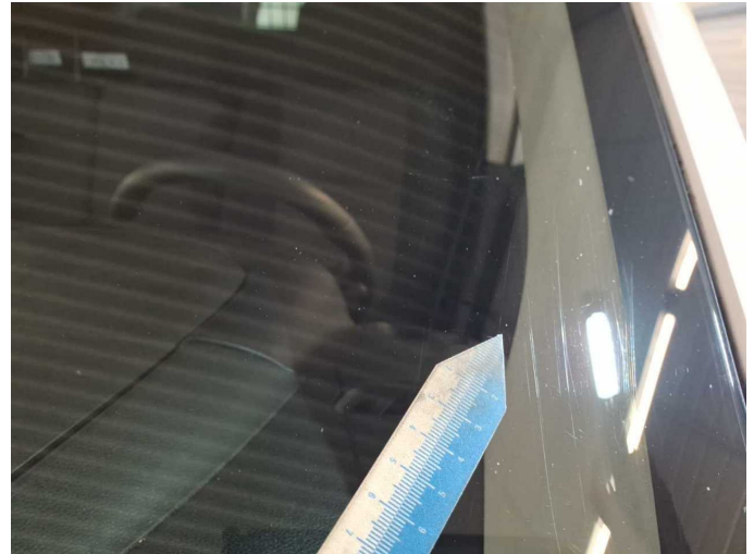
Damage 1: Vehicle glazing: Windscreen - Scratch(es) - No deduction
