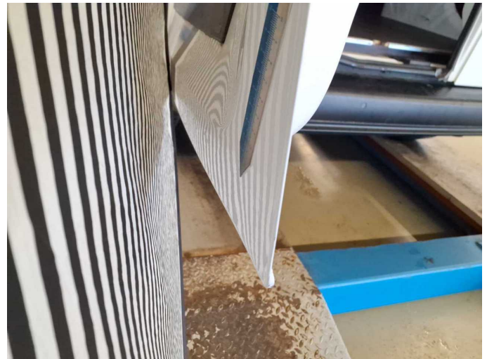
Damage 19: Boot lid / rear door: Rear door - left side - Deformed - Repair and paint
