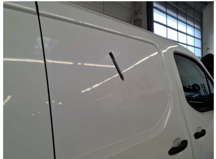
Damage 17: Sliding door, right: Sliding door (wellig) - Unprofessionally repaired - Repair and paint
