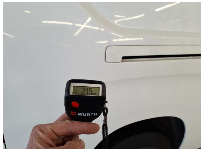
Side panel - rear right side: 215 µm
