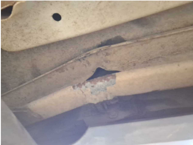
Damage 11: Rear of vehicle: Crossmember - Deformed - Replace
