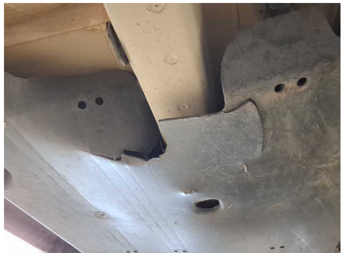
Damage 9: Body: Underbody panelling (rechts + links) - Broken / torn - Replace
