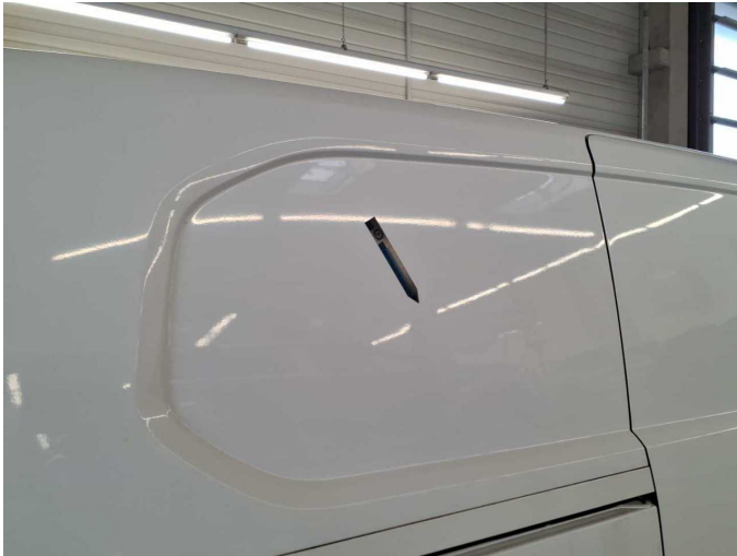
Damage 18: Side panel - rear right side: Side panel (wellig) - Unprofessionally repaired - Repair and paint
