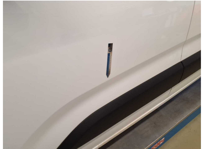
Damage 4: Door - front left side: Door - dent(s) - Smart repair
