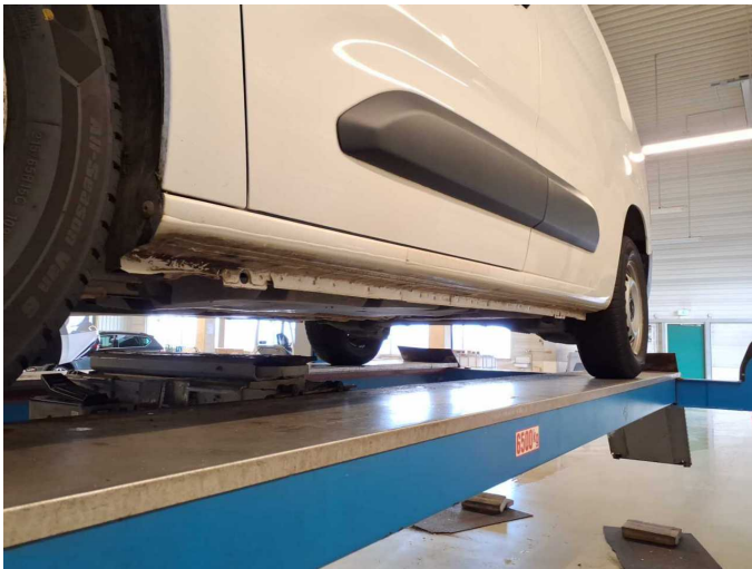
Damage 13: Sill - left side: Sill - Deformed - Repair and paint
