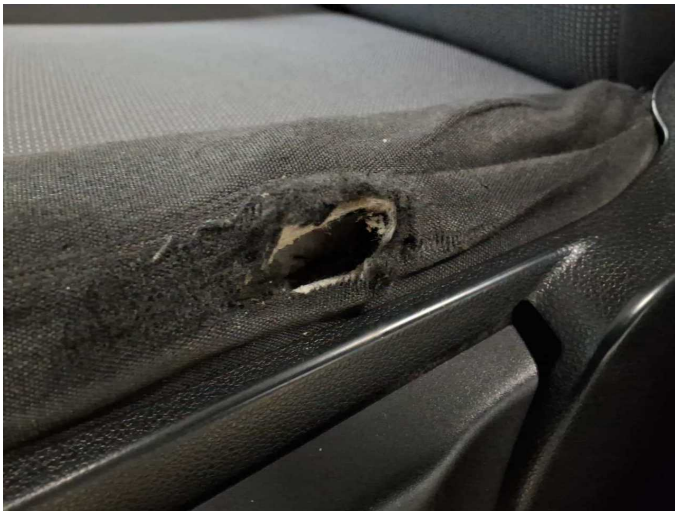
Damage 20: Seat - front: Seat cover - left side (inkl. Polster) - Broken / torn - Replace
