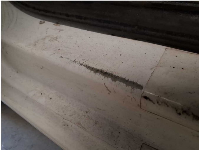
Damage 6: Sill - left side: Sill - Scratched - Smart repair
