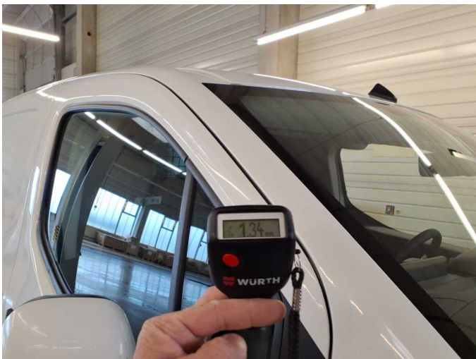
Roof rail - right side: 1,340 µm
