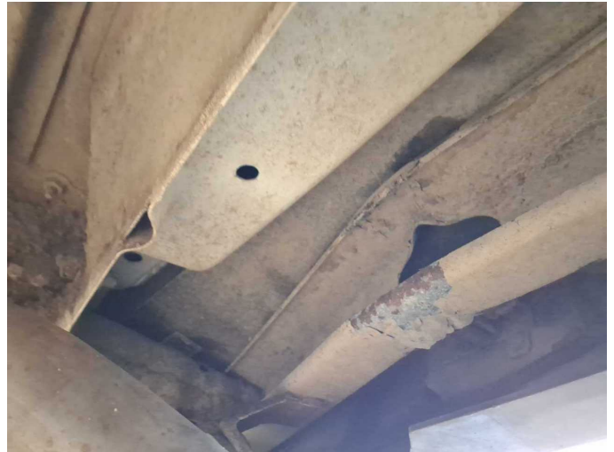
Damage 11: Rear of vehicle: Crossmember - Deformed - Replace
