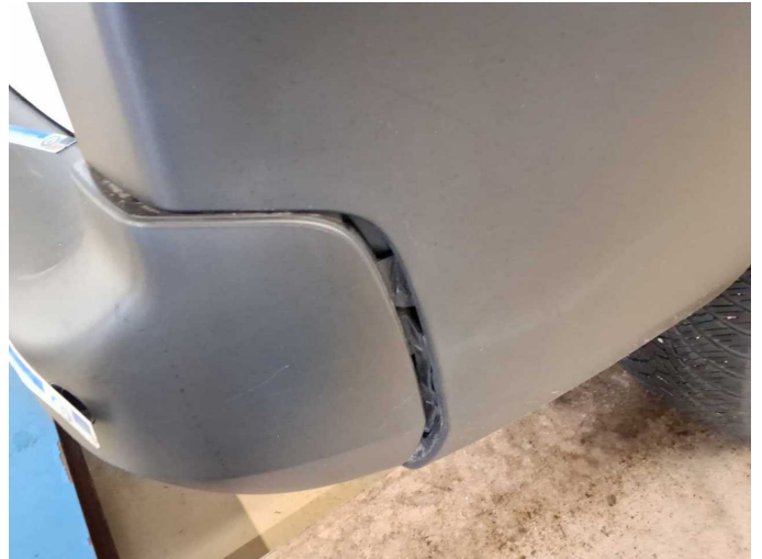
Damage 15: Rear bumper: Bumper with Parktronic - Deformed - Replace
