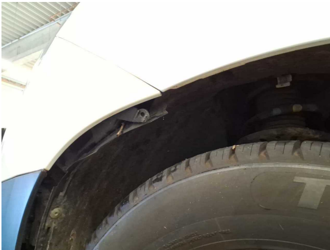
Damage 8: Mudguard - left side: Inner mudguard - Broken / torn - Replace
