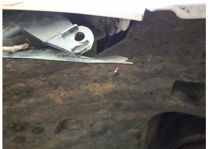
Damage 8: Mudguard - left side: Inner mudguard - Broken / torn - Replace
