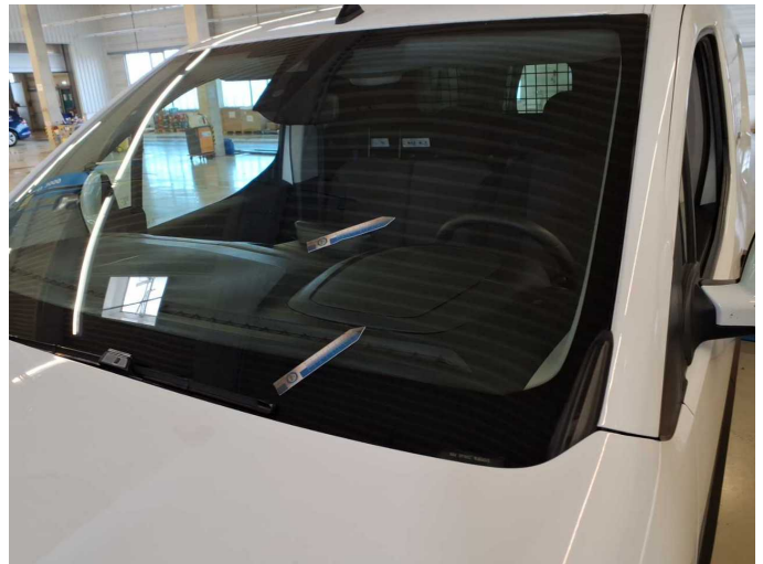
Damage 1: Vehicle glazing: Windscreen - Scratch(es) - No deduction
