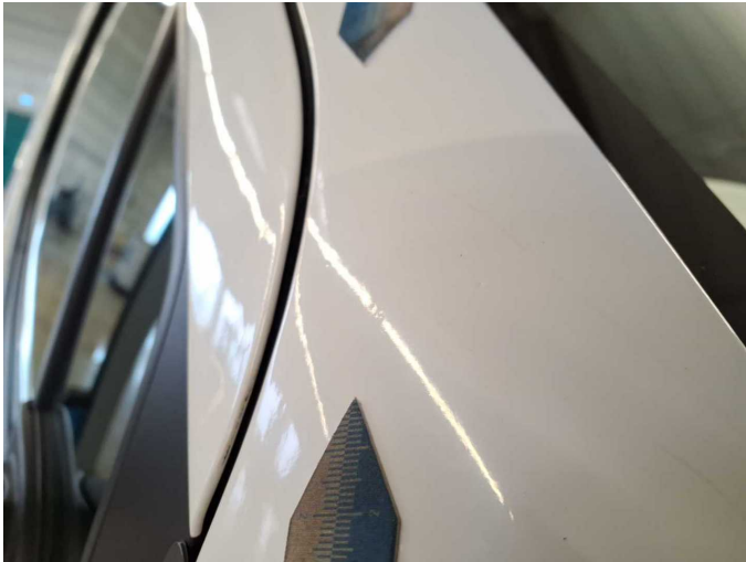
Damage 12: Roof: Roof rail - right side (A-Säule Lackeinschlüsse) - Unprofessionally repaired - Repair and paint
