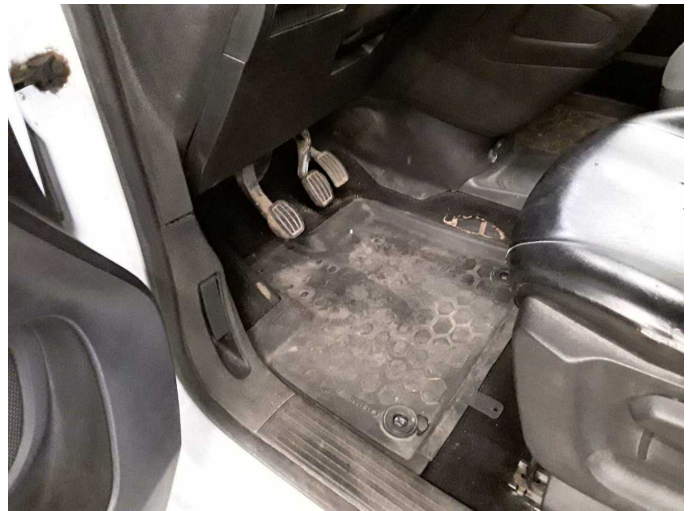
Damage 7: Trim / covers: Floor covering - front left side - Damaged - Loss in value
