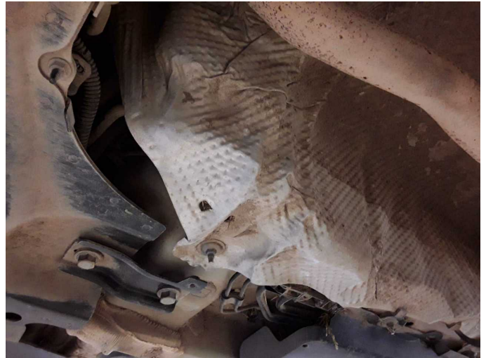
Damage 6: Exhaust system: Heat shield - Deformed - Replace
