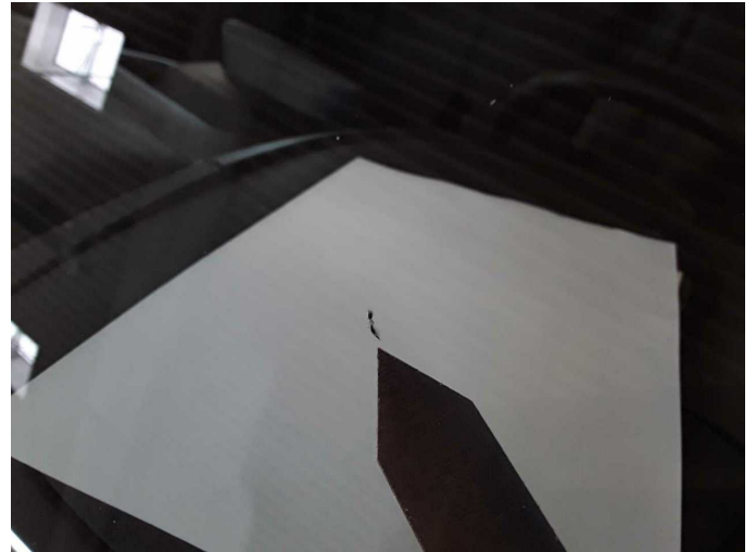
Damage 15: Vehicle glazing: Windscreen with rain sensor (Rißbildung) - Stone chips - Replace
