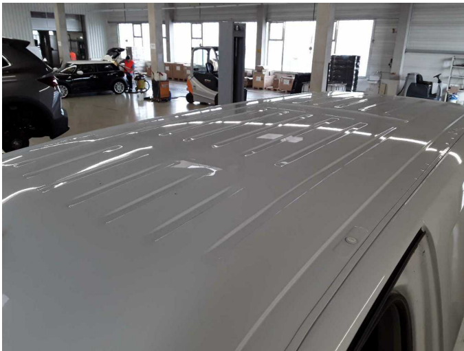
Damage 10: Roof: Roof - dent(s) - Smart repair
