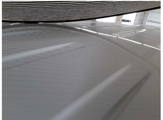
Damage 10: Roof: Roof - dent(s) - Smart repair
