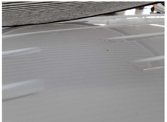
Damage 10: Roof: Roof - dent(s) - Smart repair
