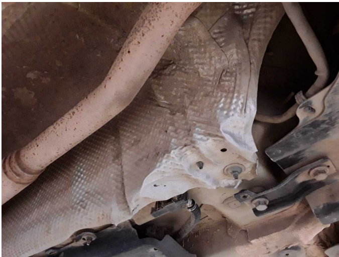
Damage 6: Exhaust system: Heat shield - Deformed - Replace
