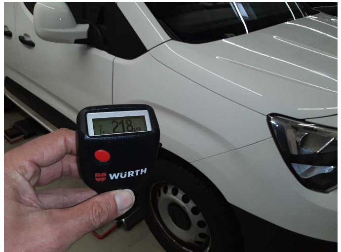
Mudguard - right side: 218 µm
