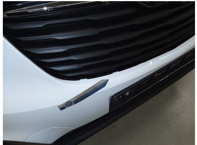
Damage 1: Front bumper: Air-inlet grille - Loose - Diagnosed and repair if necessary
