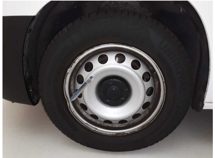
Damage 5: Wheel / tyres: Wheel rim - front left side - Deformed - Replace
