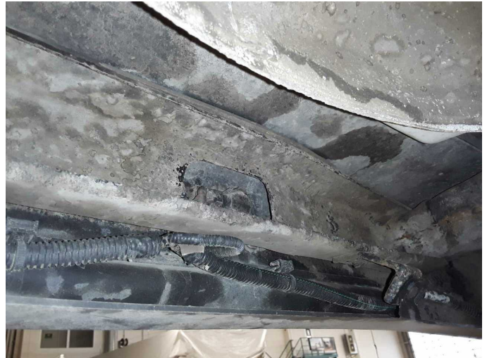
Damage 7: Rear bumper: Support - Deformed - Replace
