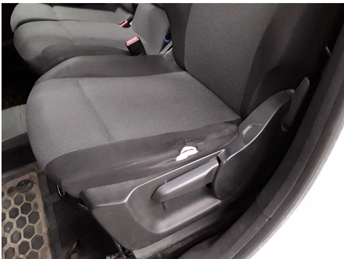
Damage 8: Seat - front: Seat upholstery - left side - Broken / torn - Replace
