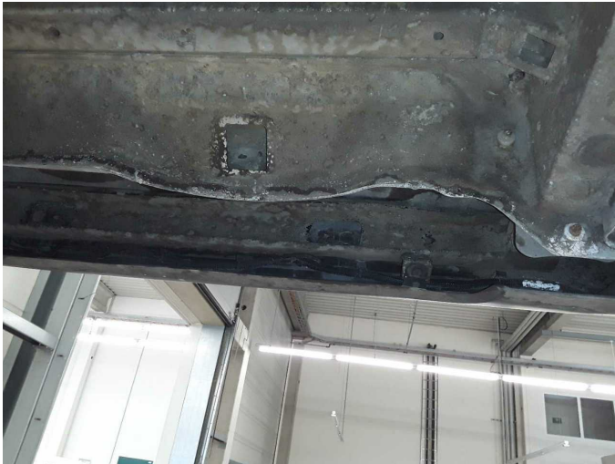
Damage 7: Rear bumper: Support - Deformed - Replace
