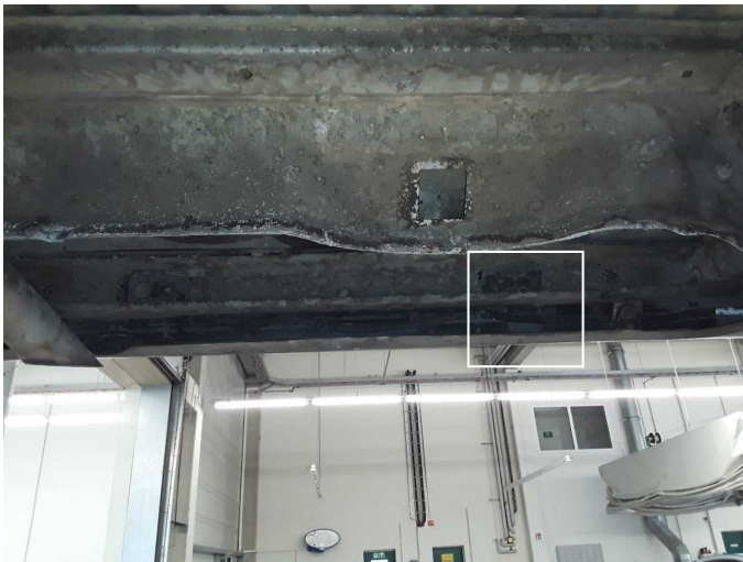
Damage 7: Rear bumper: Support - Deformed - Replace
