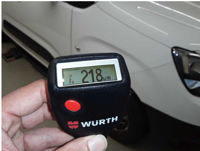
Mudguard - right side: 218 µm
