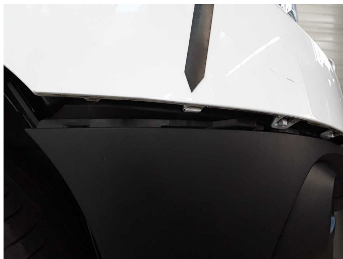
Damage 2: Front bumper: Bumper with Parktronic (Unterteil) - Loose - Repair
