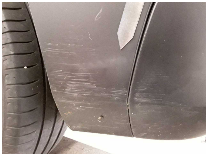
Damage 1: Rear bumper: Bumper with Parktronic - Scratched - Loss in value
