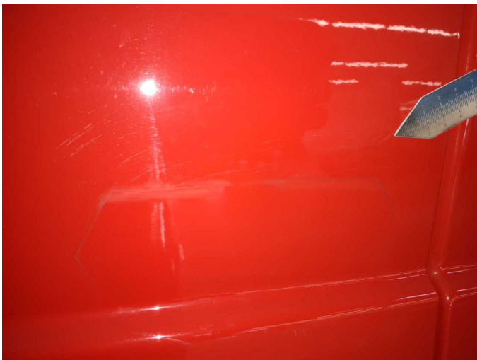
Damage 6: Boot lid / rear door: Rear door - left side - Scratch(es) - Smart repair
