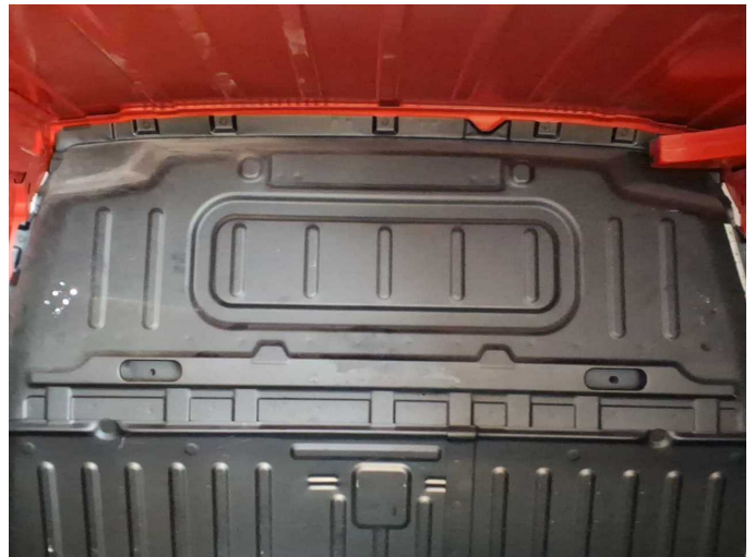
Damage 9: Body: Partition wall (Oberteil) - Differs from the original configuration - Loss in value
