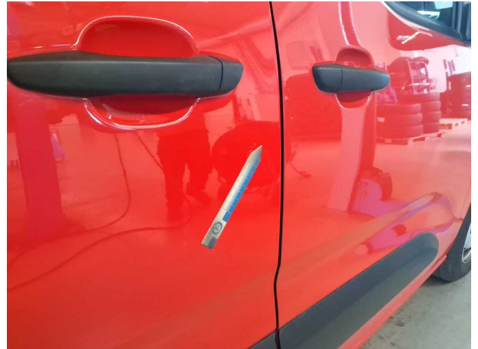
Damage 5: Sliding door, right: Sliding door - dent(s) - Smart repair
