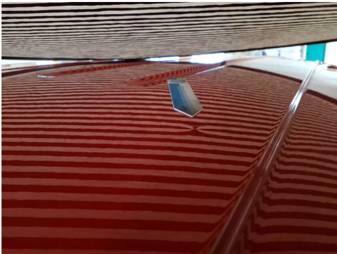
Damage 3: Roof: Roof - dent(s) - Smart repair
