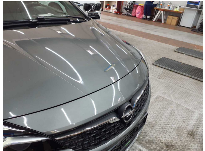
Damage 3: Bonnet: Bonnet - dent(s) - Smooth repair work
