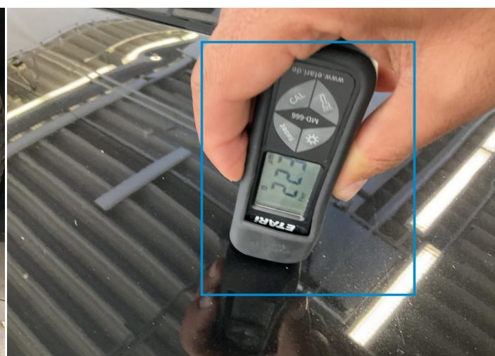
12. Hood Paint / Poor Previous Repair -
