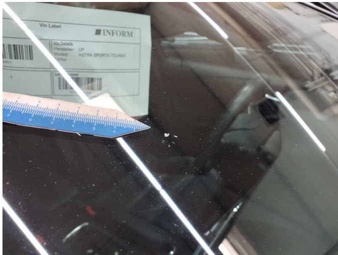
Damage 1: Vehicle glazing: Windscreen - Stone chips - No deduction
