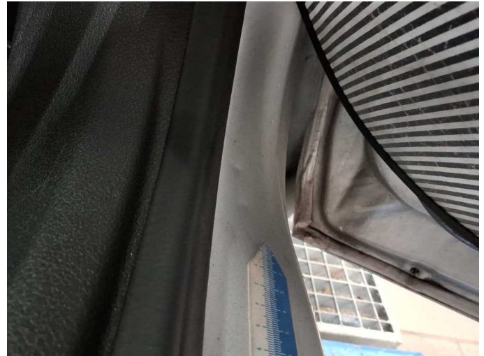
Damage 7: Sill - right side: Sill - dent(s) - Smart repair
