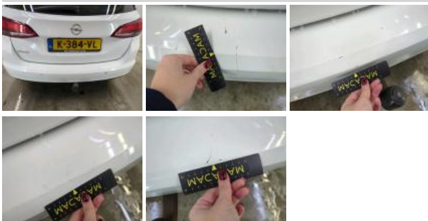
Parking sensor R, Deformed / Strained, Replace
