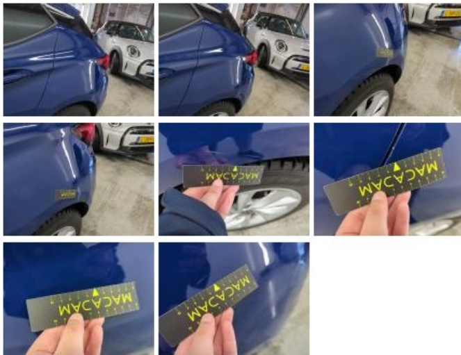
Outer door handle RL, Scratch(es), Repair and paint (complete)
