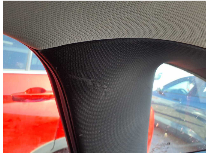
Damage 2: Trim / covers: C-pillar - trim - interior, right side - Scratch(es) - Loss in value
