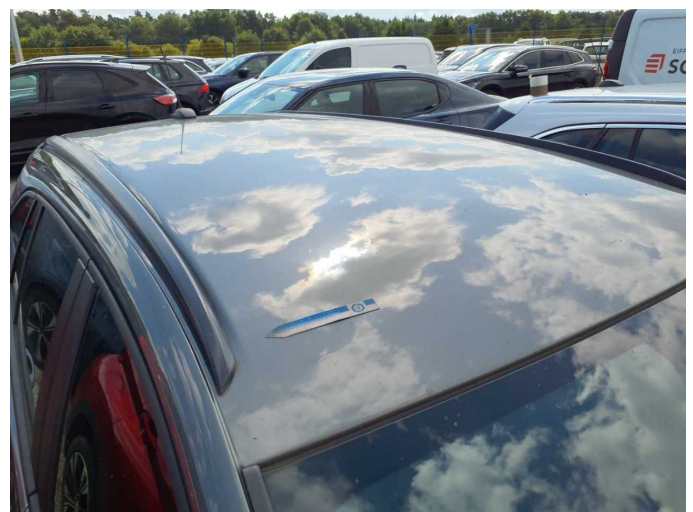
Damage 11: Roof: Roof - Deformed - Repair and paint
