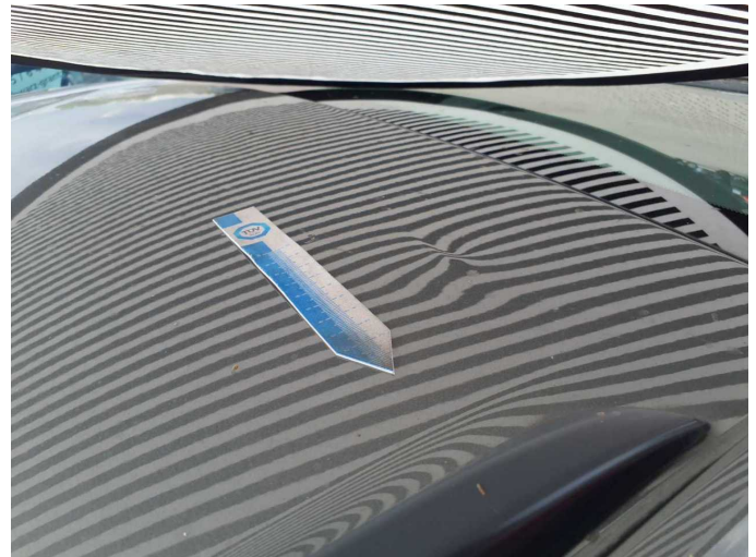
Damage 11: Roof: Roof - Deformed - Repair and paint
