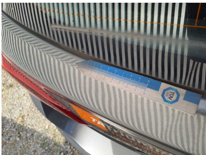
Wear and tear 4: Boot lid / rear door: Boot lid - dent(s) - No deduction
