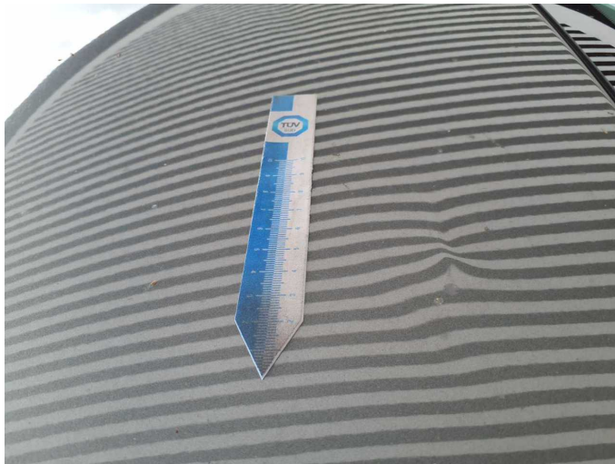
Damage 11: Roof: Roof - Deformed - Repair and paint
