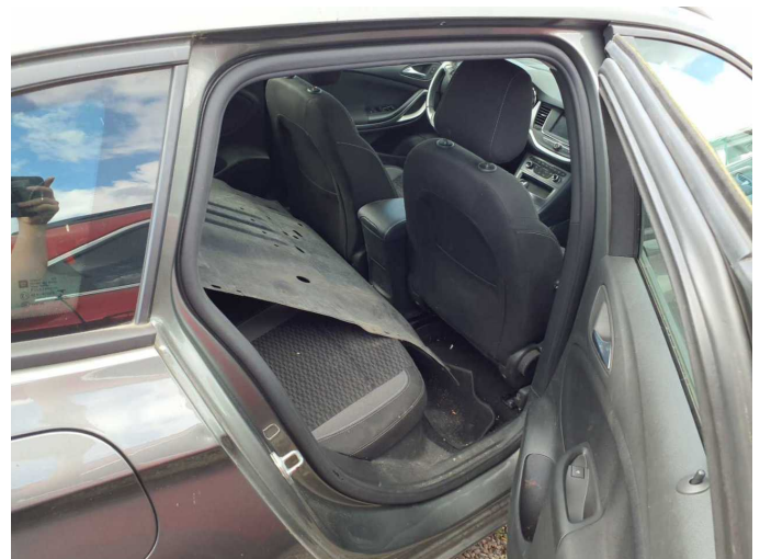
Damage 6: Door - rear right side: Door seal - Damaged - Replace
