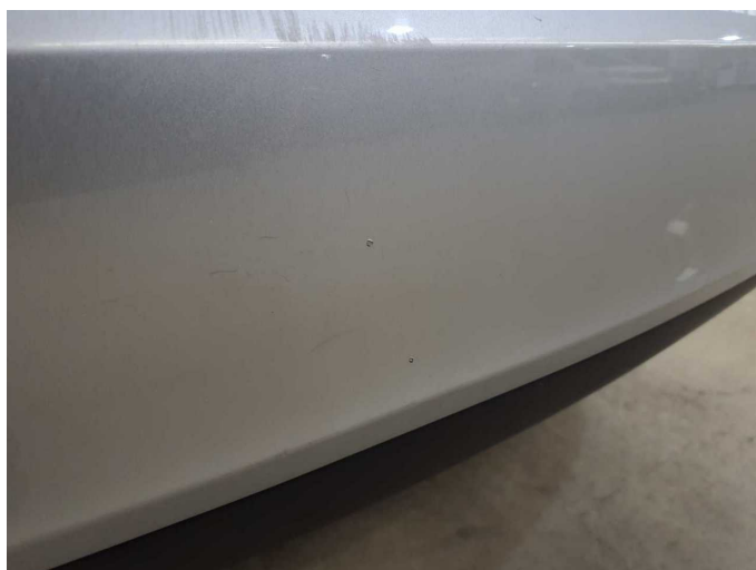
Damage 2: Rear bumper: Rear bumper - Scratch(es) - Paint
