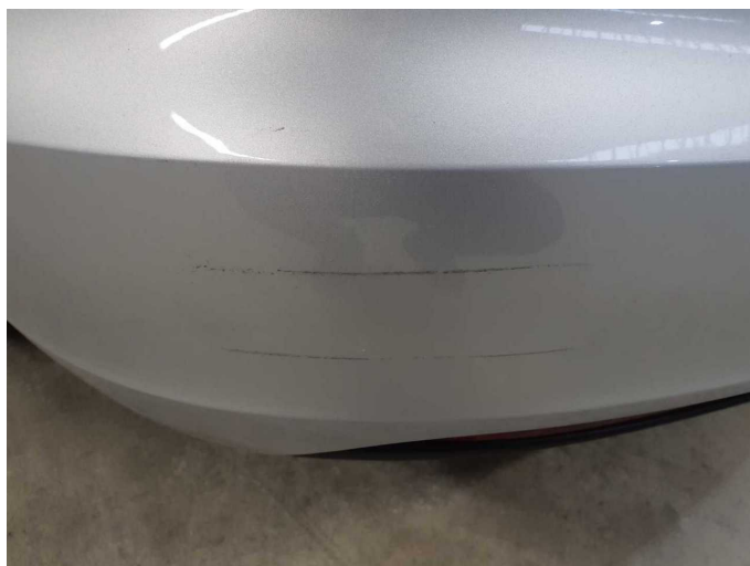
Damage 2: Rear bumper: Rear bumper - Scratch(es) - Paint
