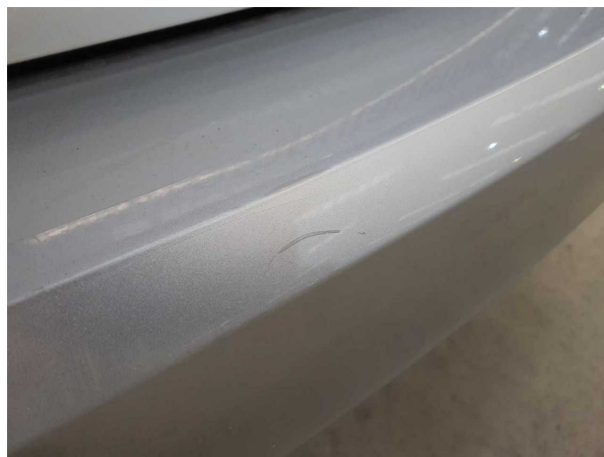
Damage 2: Rear bumper: Rear bumper - Scratch(es) - Paint
