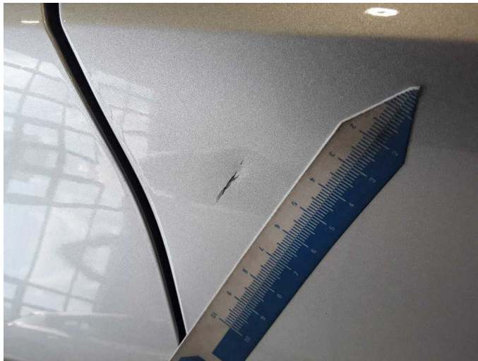
Damage 2: Door - front right side: Door - Dent / paintcoat damage - Smart repair
