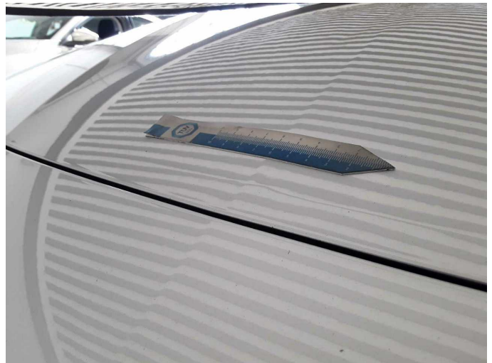
Damage 4: Bonnet: Bonnet - Deformed - Repair and paint
