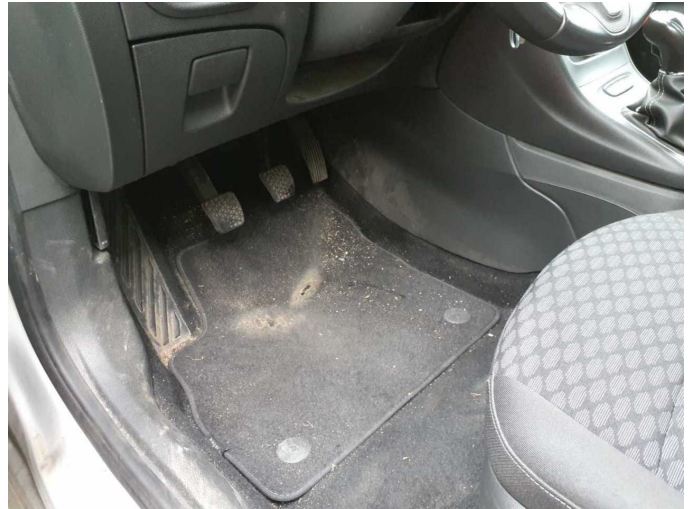
Damage 1: Trim / covers: Floor mats - Holes - Replace
