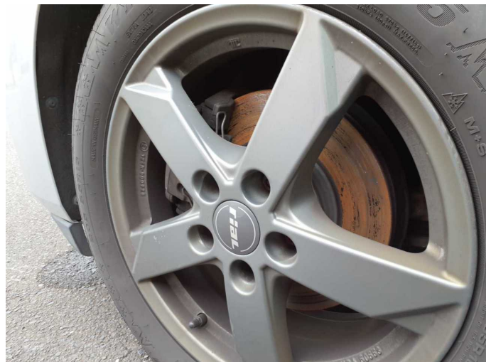
Damage 10: Braking system: Brake discs and brake pads - front (Tragbild mangelhaft) - Corrosion - Replace
