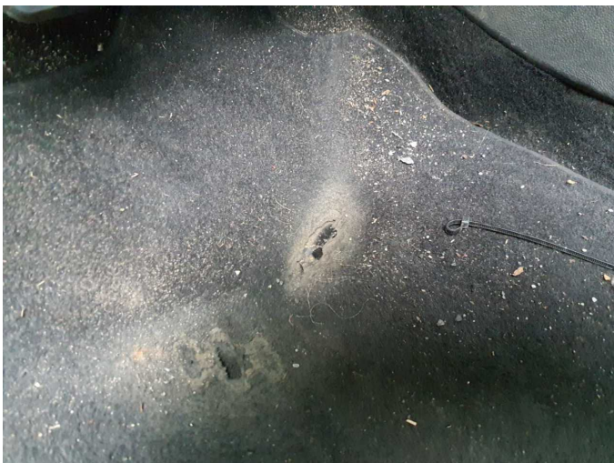
Damage 1: Trim / covers: Floor mats - Holes - Replace
