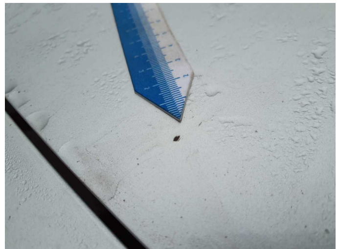
Damage 13: Bonnet: Bonnet (Korrosion) - Stone chips - Repair and paint
