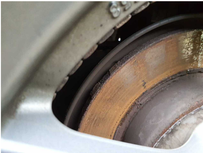
Damage 9: Braking system: Brake discs and pads - rear (Tragbild mangelhaft) - Corrosion - Replace
