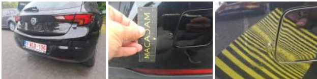
Wing RR, Dent(s), Repair and paint (complete)
