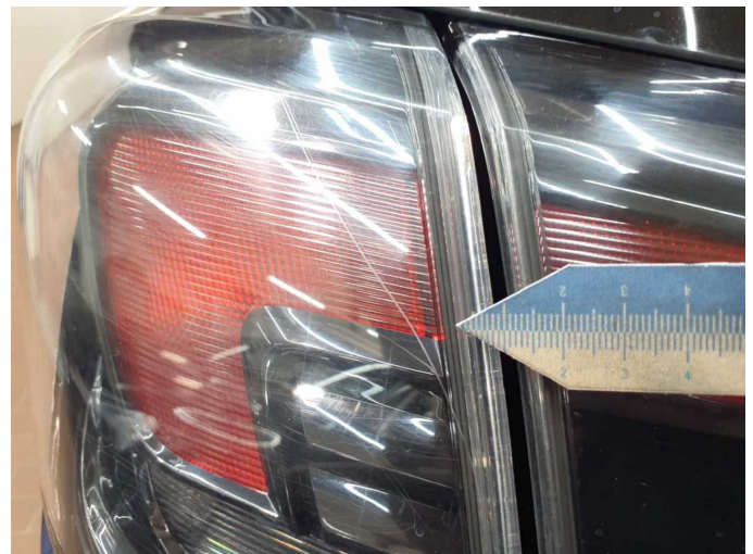
Wear and tear 4: Tail light: Tail lamp - left side - Scratch(es) - No deduction
