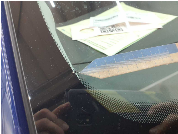
Damage 8: Vehicle glazing: Windscreen - Stone chips - Replace
