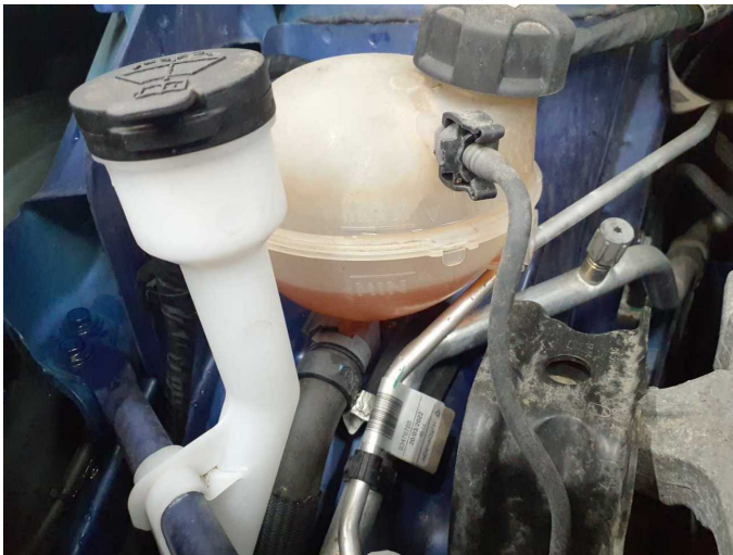
Damage 6: Engine cooling: Coolant - Missing - Perform diagnosis
