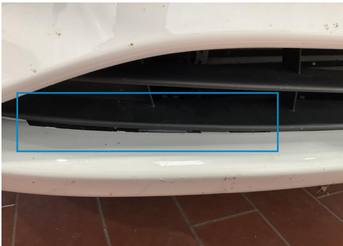
2. Blade/spoiler / Front Bodywork / Breakage -
