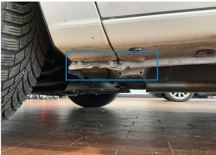
4. Rocker Panel / Center Left Bodywork / Dent / Dent -
