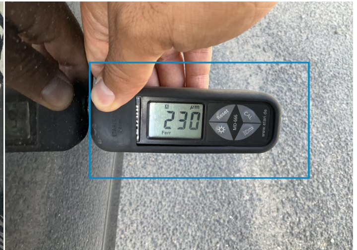
2. Door / Front Right Paint / Poor Previous Repair -
