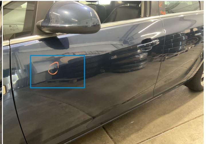
4. Door / Front Left Bodywork / Dent / Dent -
