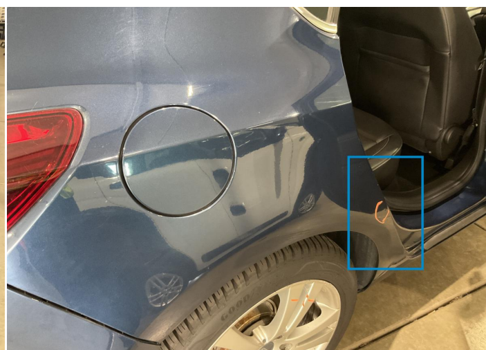
10. Side Panel / Back Right Bodywork / Dent / Dent -
