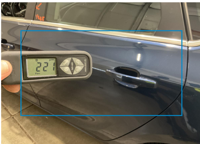
7. Door / Back Left Paint / Poor Previous Repair -
