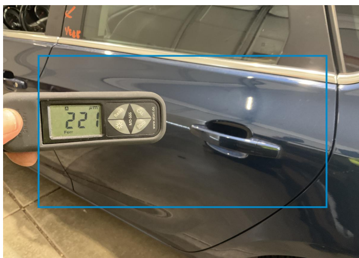
7. Door / Back Left Paint / Poor Previous Repair -
