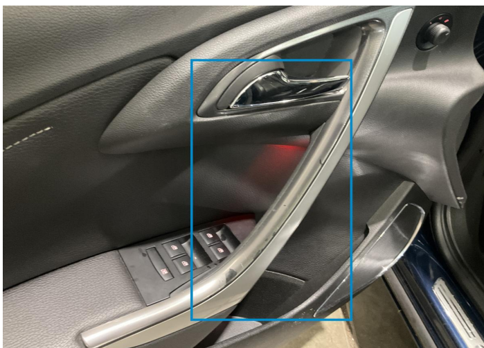
5. Panel Filling / Front Left Interior / Scratched -
