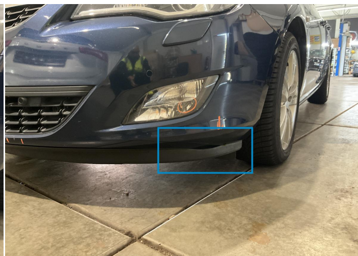
2. Blade/spoiler / Front Bodywork / Breakage / Hole -
