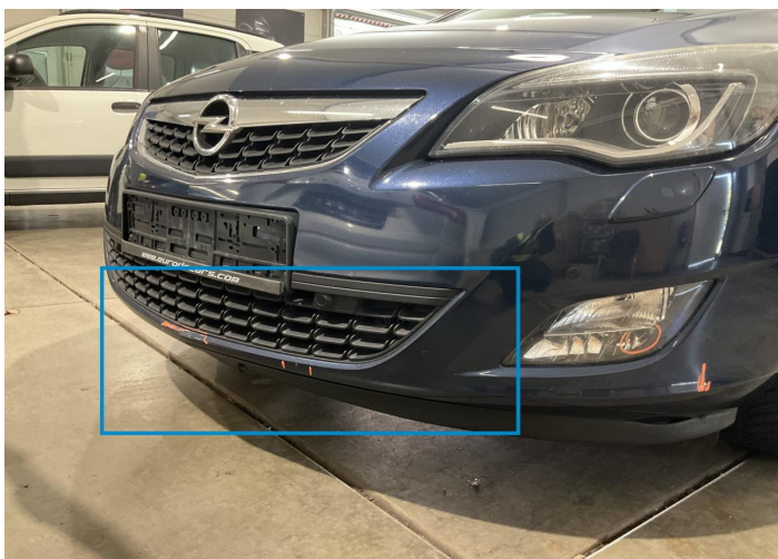
1. Bumper / Front Bodywork / Breakage / Hole -
