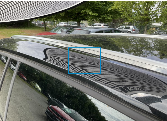
1. Roof Bodywork / Dent / Dent -
