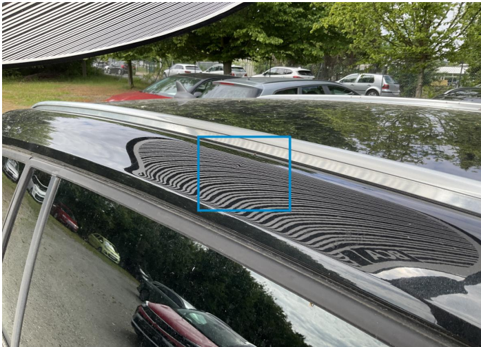
1. Roof Bodywork / Dent / Dent -
