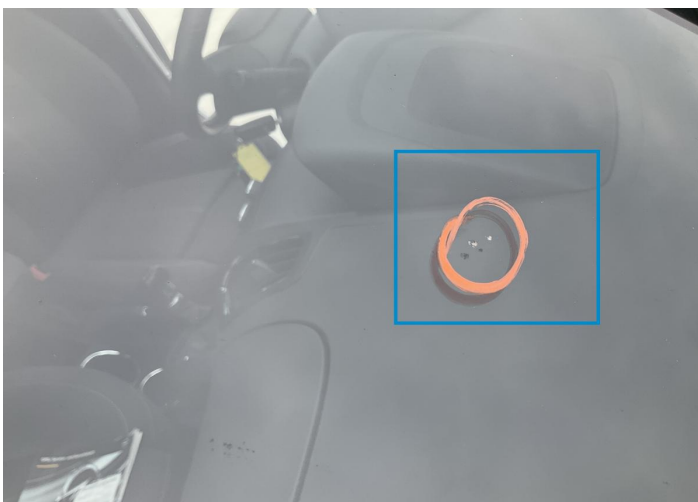
5. Windshield / Front Paint / Chipping -
