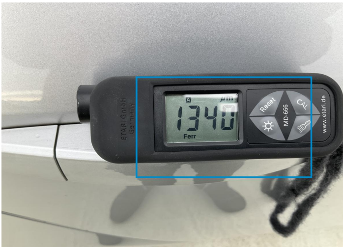
1. Fender / Back Right Paint / Poor Previous Repair -
