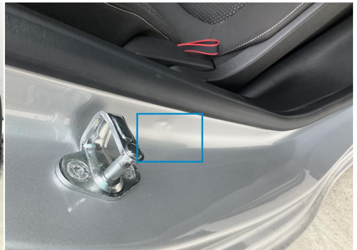
2. Pillar / Back Right Bodywork / Dent / Dent -
