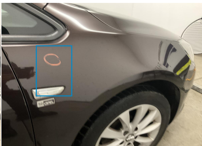
10. Fender / Front Right Bodywork / Dent / Dent -
