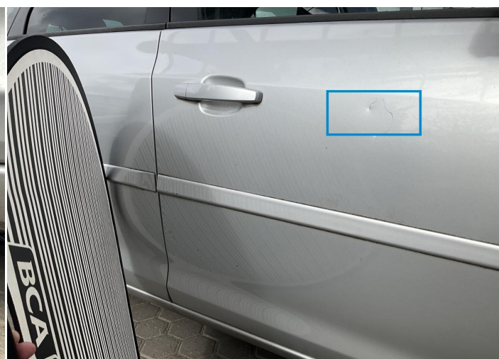
10. Door / Front Right Bodywork / Dent / Dent -
