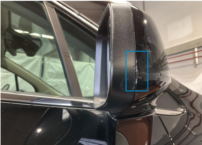
10. Mirror / Front Right Paint / Stone Chip -
