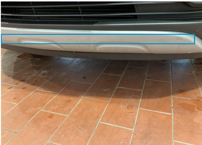
1. Blade/spoiler / Front Paint / Scratch / Line -
