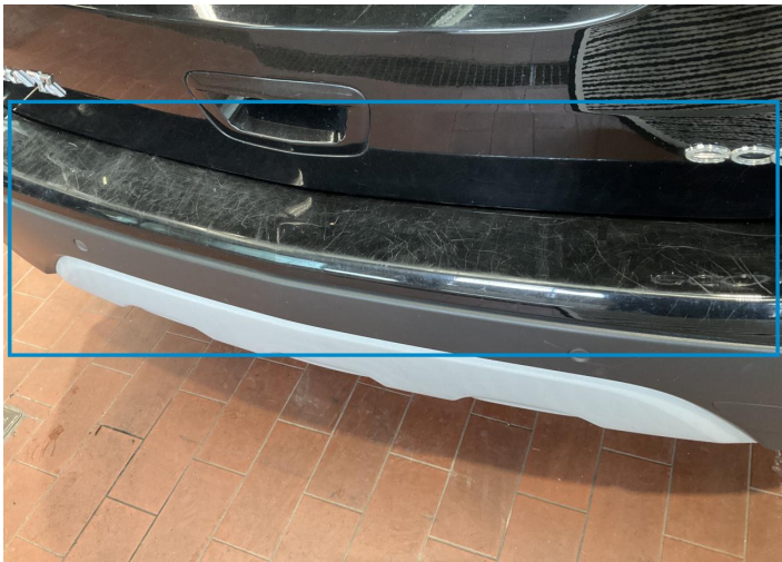
5. Bumper / Back Paint / Scratch / Line -
