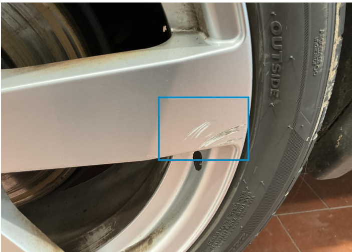
2. Rim / Front Left Out of Bodywork / Scratch -
