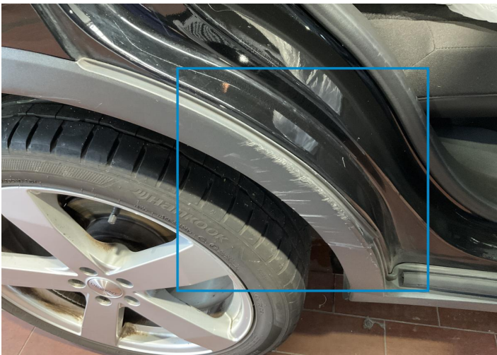
8. Wing Stick / Back Right Paint / Scratch / Scuff -
