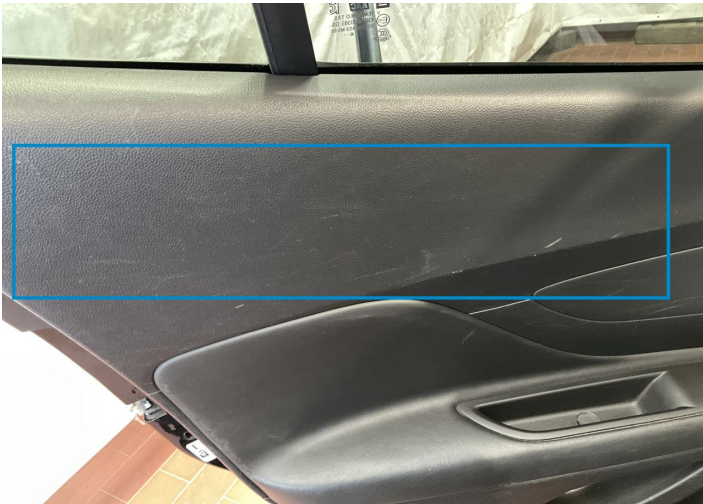
4. Panel Filling / Back Left Interior / Scratched -
