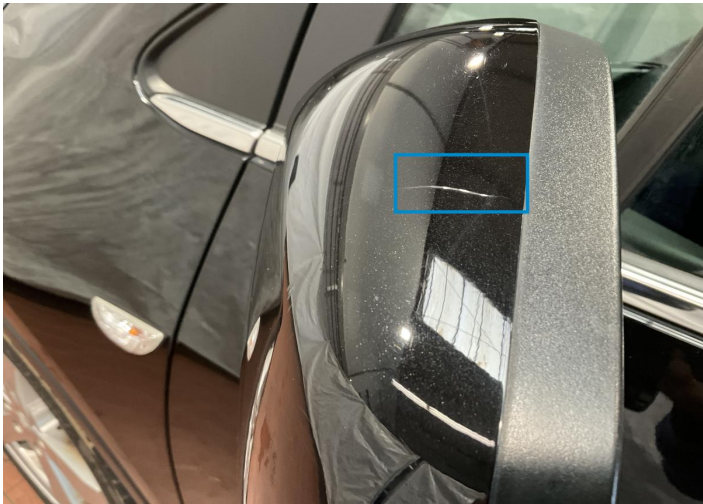
3. Mirror / Front Left Paint / Stone Chip -
