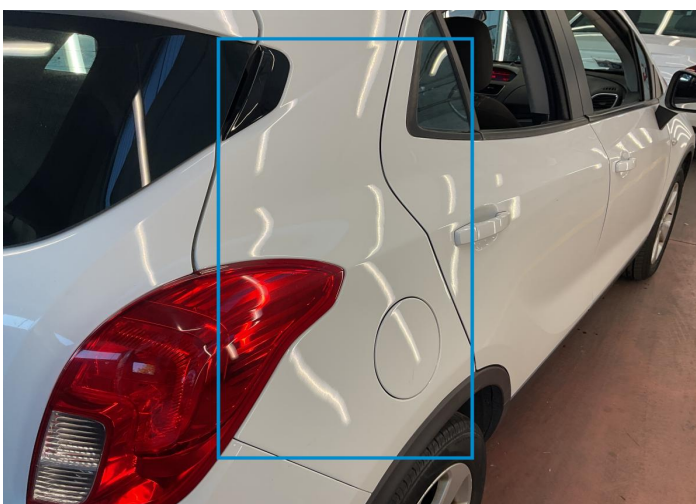
21. Fender / Back Right Bodywork / Dent / Hail Area -
