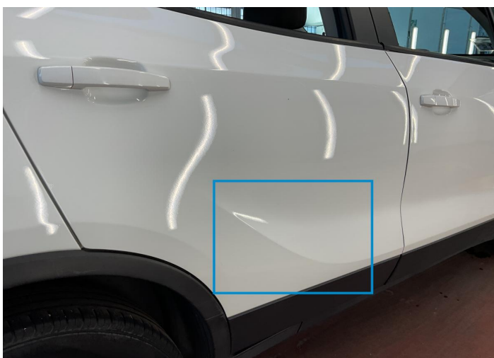
22. Door / Back Right Bodywork / Dent -
