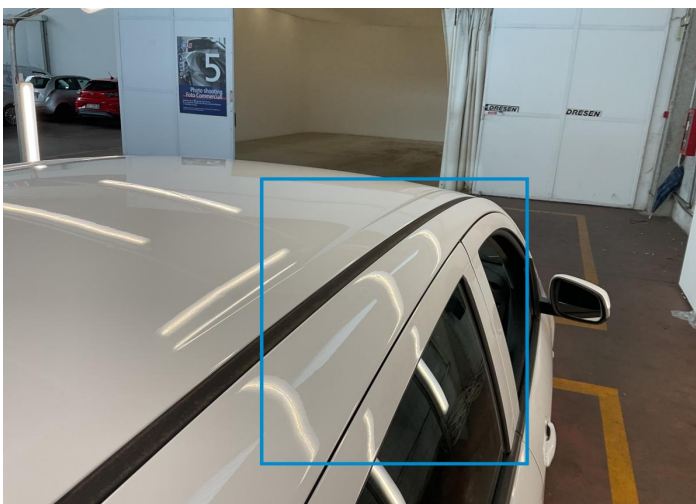
18. Pillar / Front Right Bodywork / Dent / Hail Area -
