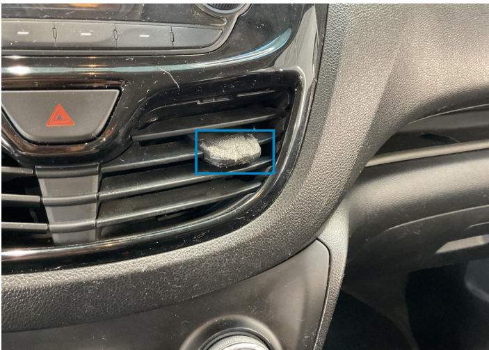
2. Aeration Grid / Front Center Interior / Broken -
