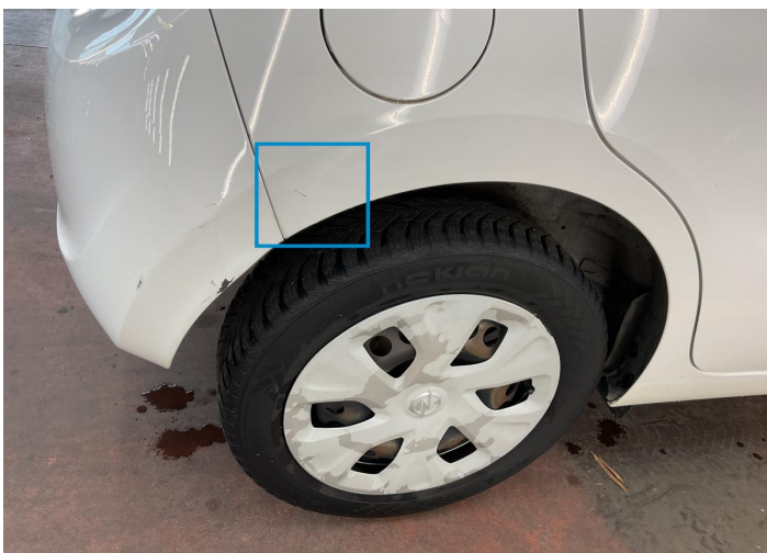
12. Fender / Back Right Bodywork / Dent -
