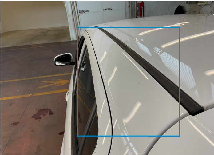
19. Pillar / Front Left Bodywork / Dent / Hail Area -
