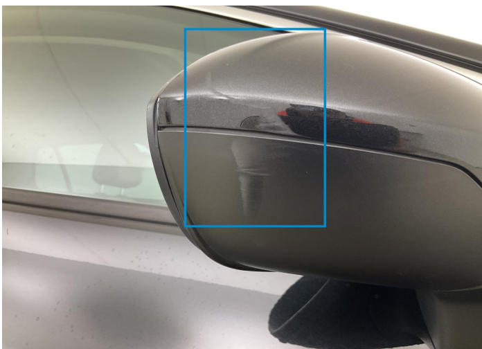
8. Mirror Shell / Front Right Paint / Scratch / Scuff -
