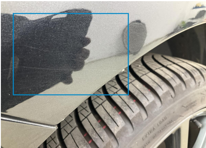
6. Side Panel / Back Right Paint / Scratch / Scuff -
