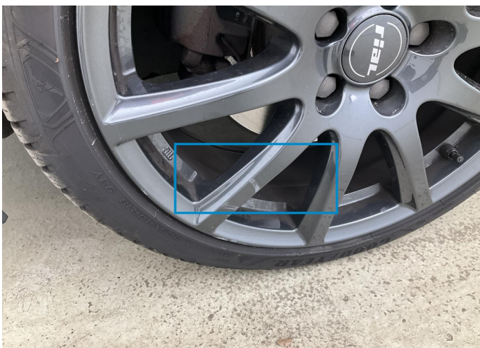
12. Rim / Front Left Out of Bodywork / Scratch -
