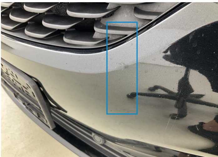
10. Bumper / Front Paint / Chipping -
