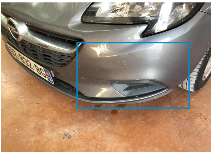
1. Shield / Front Paint / Scratch / Line -
