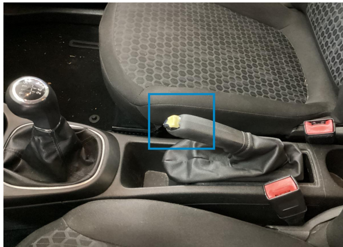
13. HandBrake Handle Interior / Ripped -
