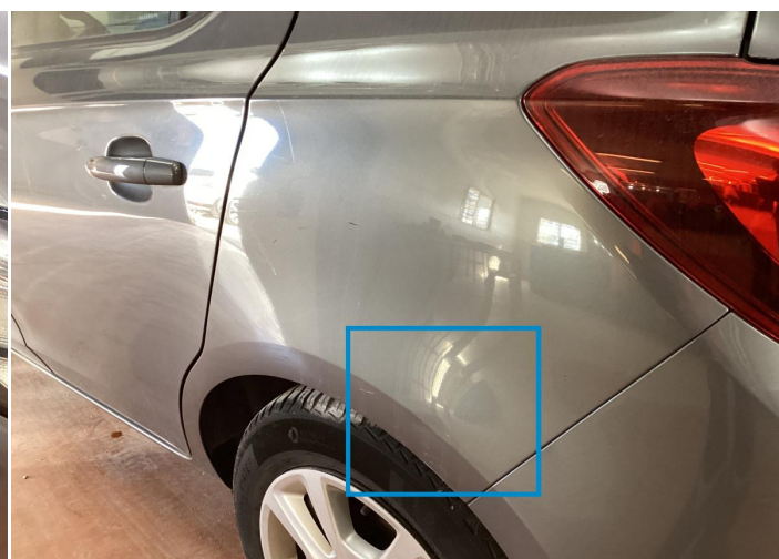
8. Fender / Back Left Bodywork / Dent / Deformation -
