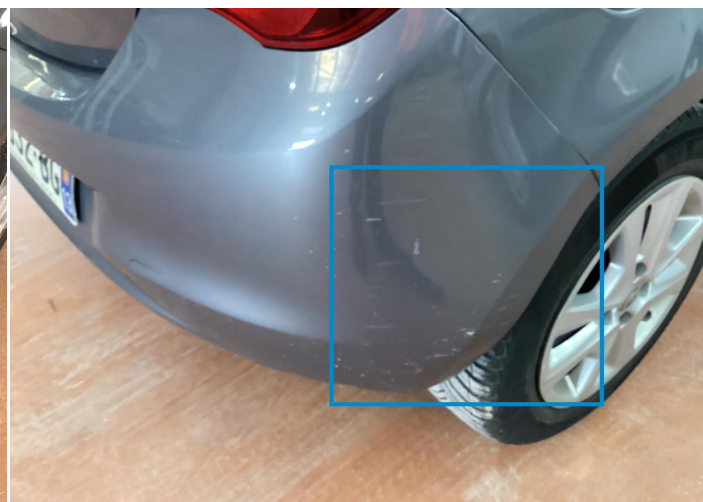
2. Shield / Back Bodywork / Dent / Deformation -
