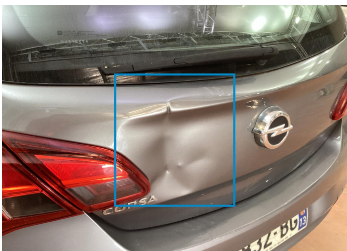
3. Tailgate Bodywork / Dent / Deformation -
