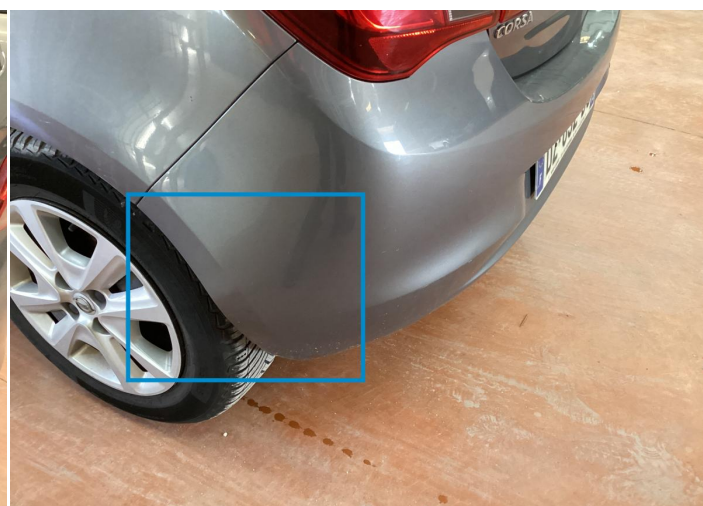
4. Shield / Back Bodywork / Dent / Deformation -
