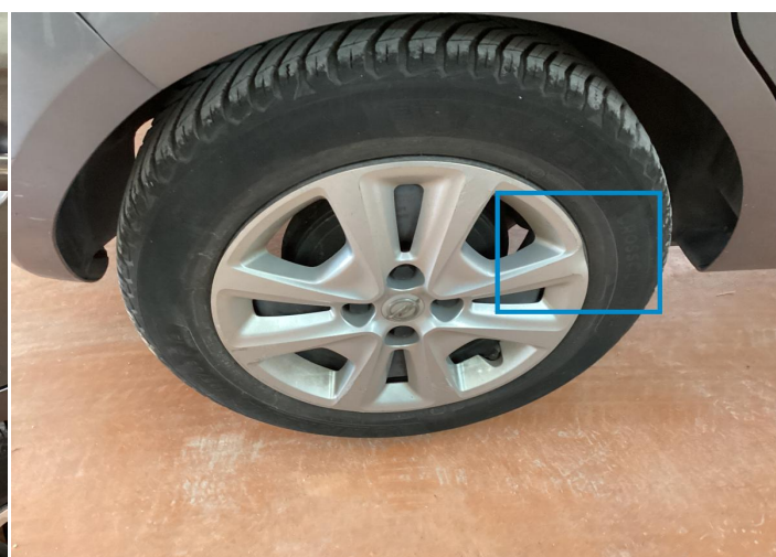
12. Hubcap / Back Right Out of Bodywork / Breakage -
