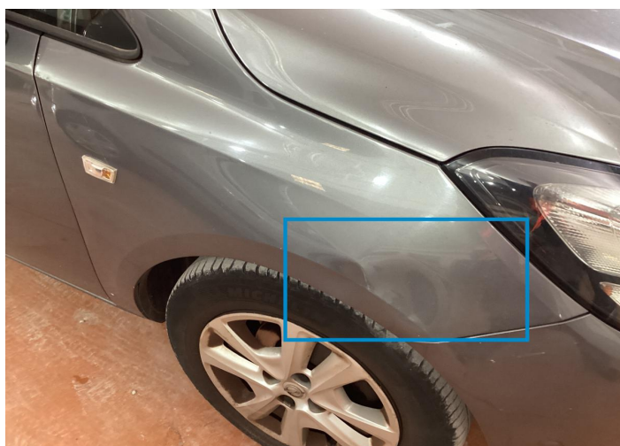
7. Fender / Front Right Bodywork / Dent / Deformation -
