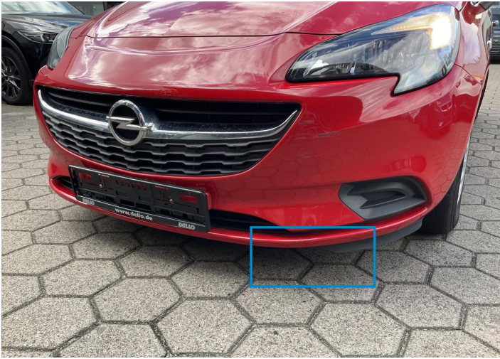
24. Bumper / Front Paint / Scratch / Scuff -
