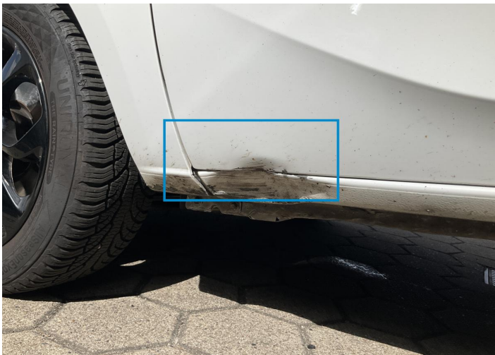
2. Door / Front Left Bodywork / Dent / Dent -
