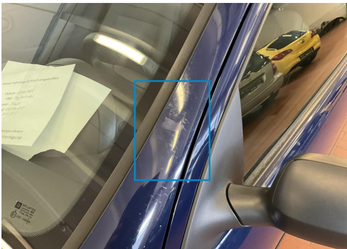
23. Pillar / Front Left Paint / Chipping -
