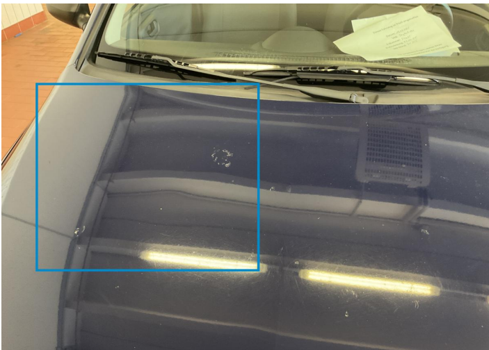
22. Hood Paint / Chemical Damage -
