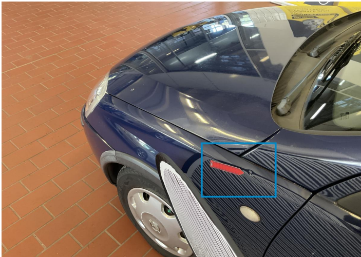
1. Fender / Front Left Bodywork / Dent / Dent -
