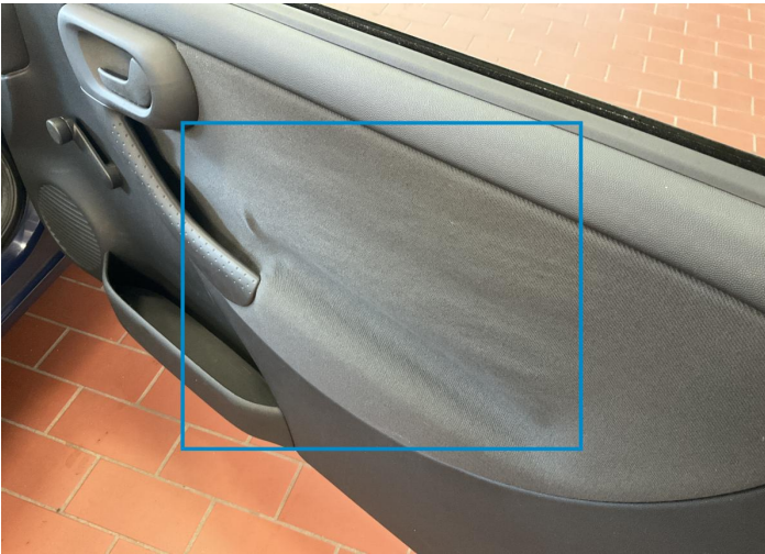
25. Panel Filling / Front Right Interior / Loose -
