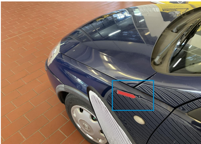
1. Fender / Front Left Bodywork / Dent / Dent -
