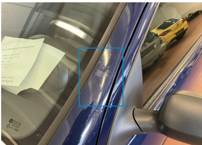
23. Pillar / Front Left Paint / Chipping -
