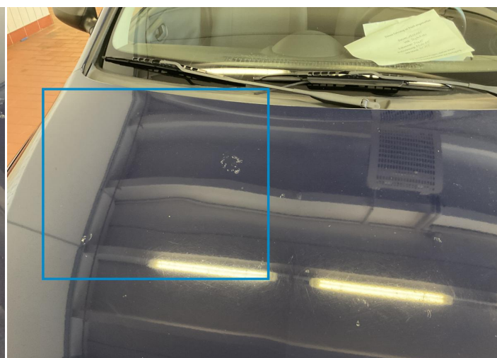
22. Hood Paint / Chemical Damage -
