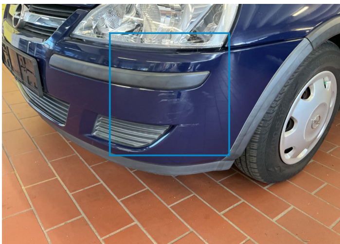
19. Bumper / Front Paint / Scratch / Scuff -
