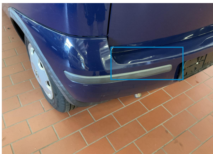
9. Bumper / Back Bodywork / Breakage / Crack -
