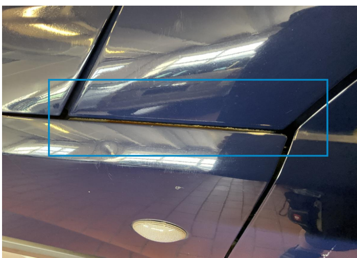
29. Pillar / Front Left Paint / Corrosion -
