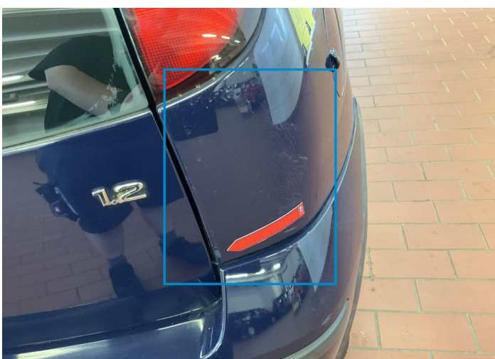
12. Fender / Back Right Paint / Scratch / Scuff -
