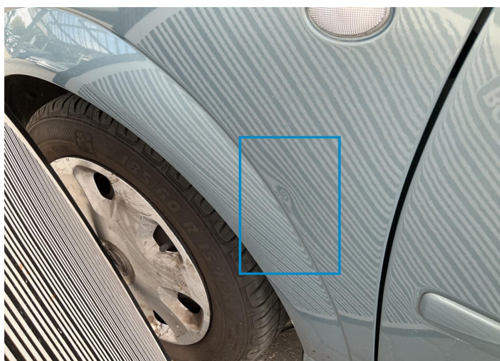
3. Fender / Front Left Bodywork / Dent / Dent -
