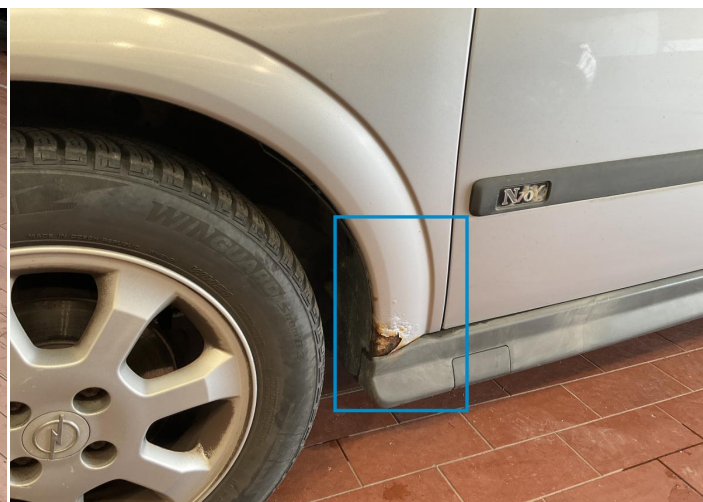
2. Fender / Front Left Paint / Corrosion -
