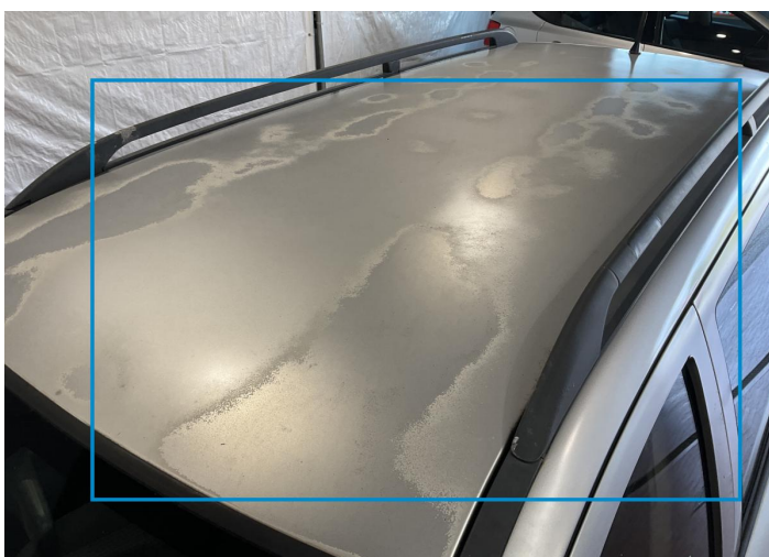
3. Roof Paint / Scratch / Scuff -
