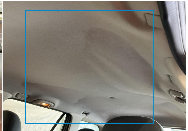
10. Roof Upholstery Interior / Loose -
