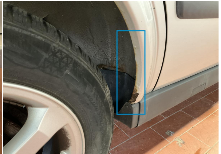
8. Side Panel / Back Right Paint / Corrosion -
