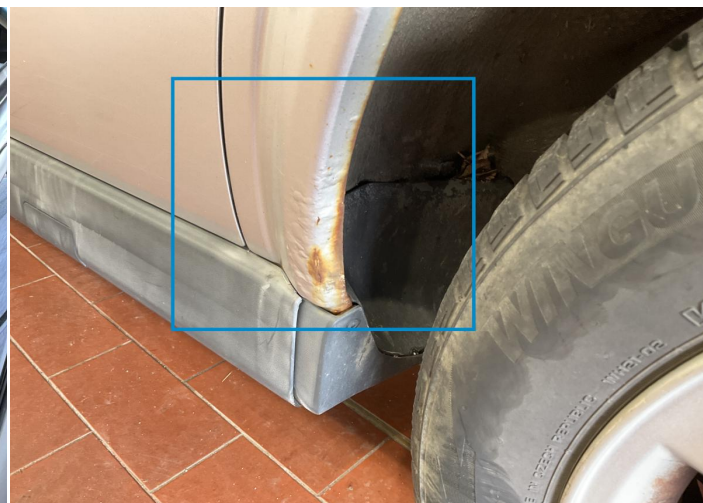
4. Side Panel / Back Left Paint / Corrosion -
