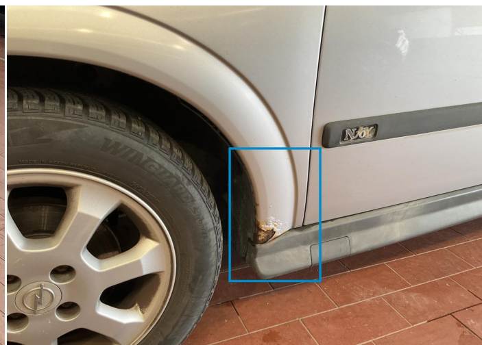
2. Fender / Front Left Paint / Corrosion -
