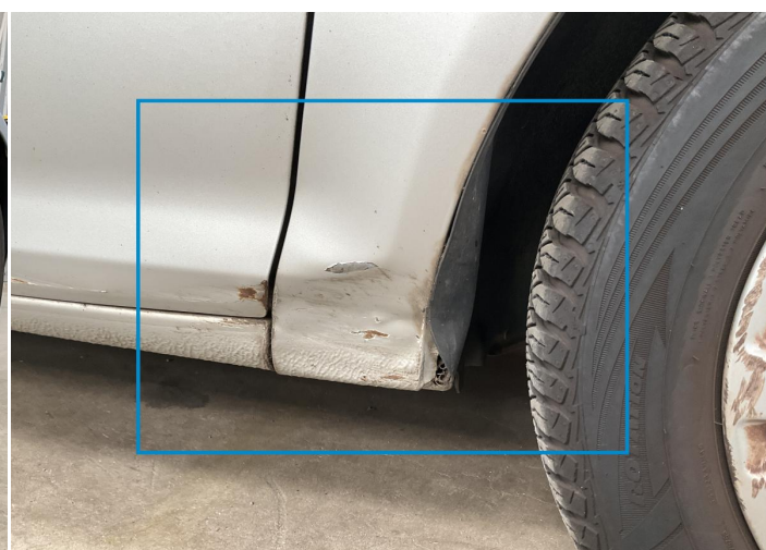
12. Fender / Front Right Bodywork / Dent / Deformation -
