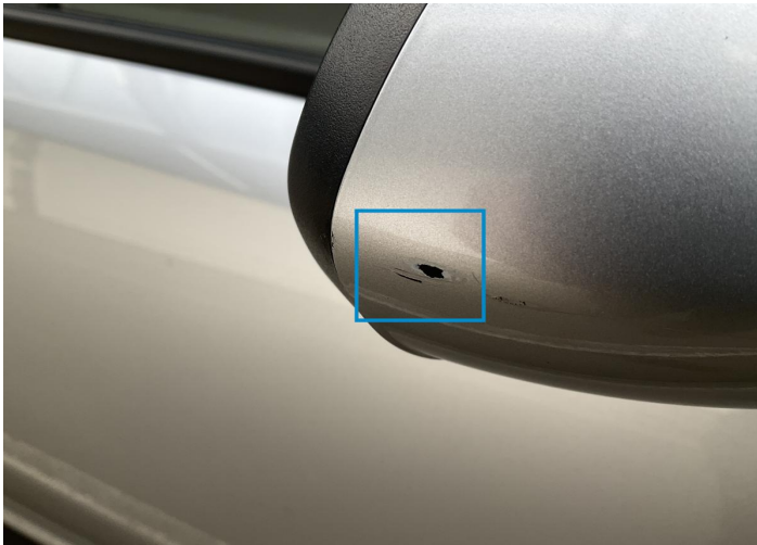
15. Mirror Shell / Front Right Paint / Scratch / Scuff -
