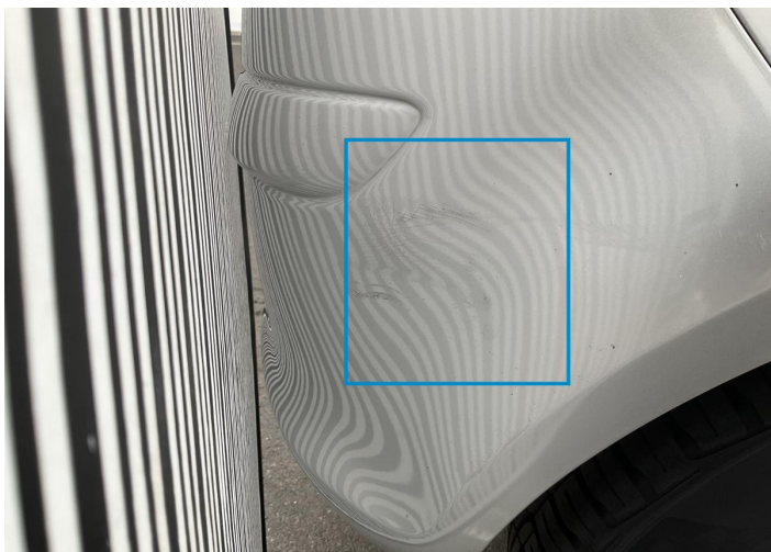
9. Bumper / Back Bodywork / Dent / Dent -
