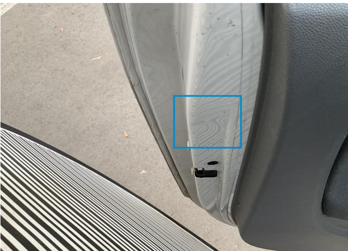
5. Door / Front Left Bodywork / Dent / Dent -
