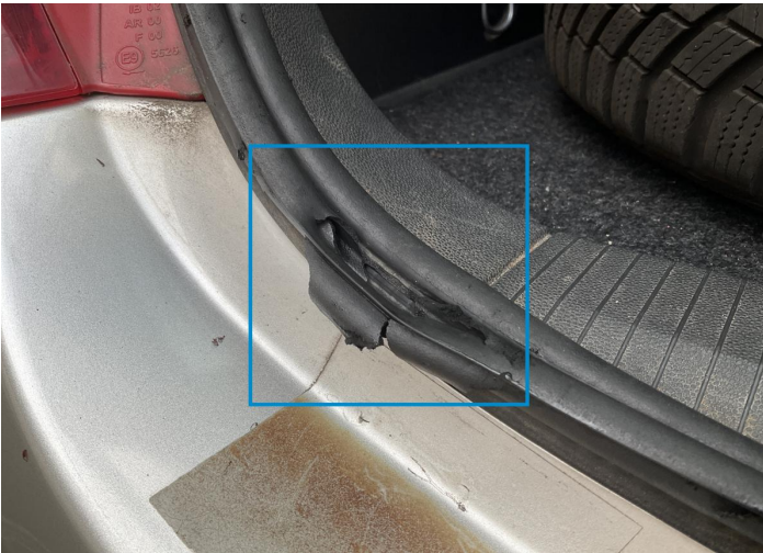
3. Luggage Space Cover / Back Interior / Ripped -
