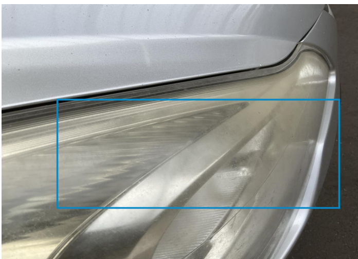
8. Front Light / Front Right Glass Break -
