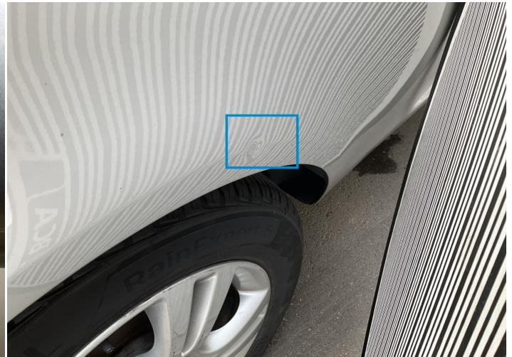
16. Side Panel / Back Right Bodywork / Dent / Dent -
