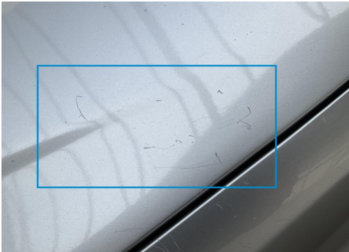
13. Hood Paint / Scratch / Scuff -
