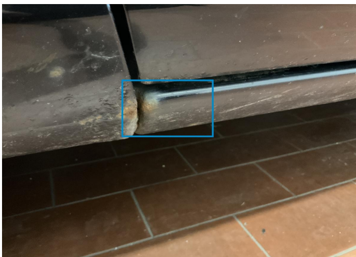
5. Rocker Panel / Center Left Paint / Scratch / Line -
