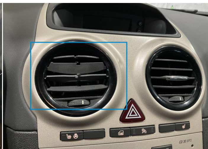
8. Aeration Grid / Front Center Interior / Broken -
