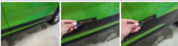
Door FR, Dent(s) and scratch(es), Light repair (medium)
