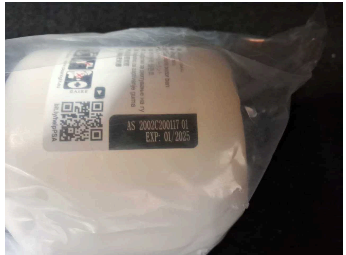
Damage 1: Equipment: Tirefit filler - Expired - Replace
