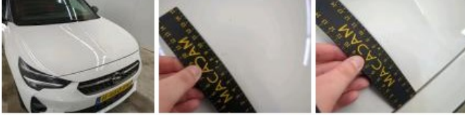
Bumper F, Scratch(es), Repair and paint (complete)
