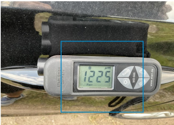
1. Door / Back Left Paint / Poor Previous Repair -
