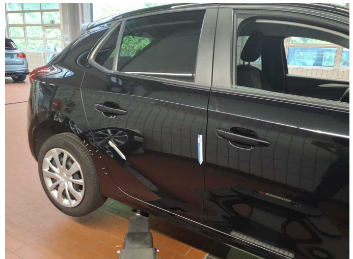
Damage 18: Door - rear right side: Door - Dent / paintcoat damage - Repair and paint
