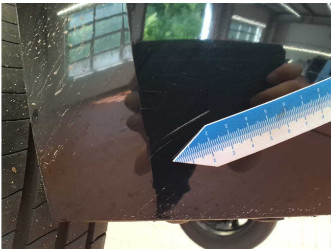
Damage 19: Rear bumper: Rear bumper - Scratch(es) - Paint
