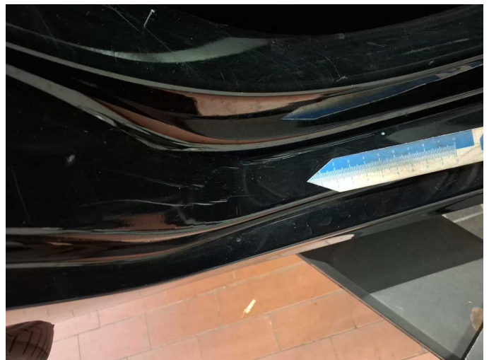
Damage 14: Side panel - rear right side: Sill - Dent / paintcoat damage - Smart repair
