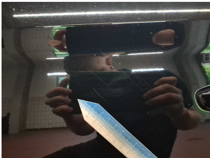
Damage 20: Door - front left side: Door - Dent / paintcoat damage - Repair and paint
