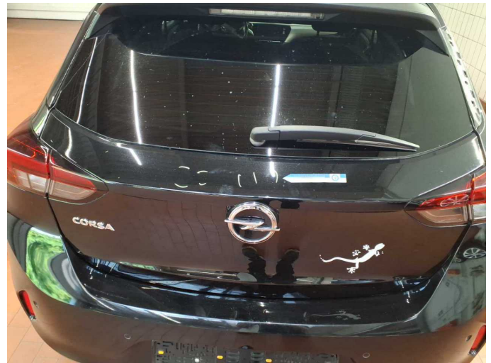
Damage 10: Boot lid / rear door: Boot lid - dent(s) - Smart repair
