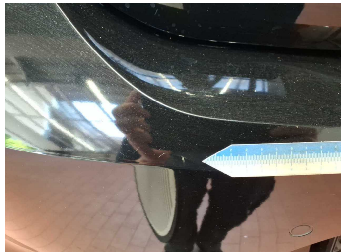
Damage 19: Rear bumper: Rear bumper - Scratch(es) - Paint
