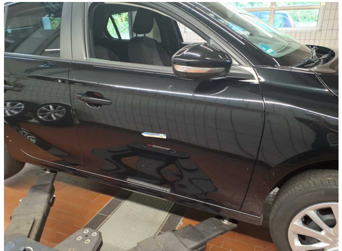
Damage 12: Door - front right side: Door - Dent / paintcoat damage - Smart repair
