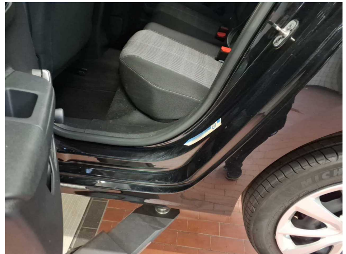
Damage 8: Side panel - rear left side: Sill - Scratch(es) - Smart repair
