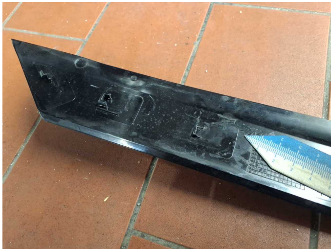
Damage 7: Side panel - rear right side: Protection strip (Hinten rechts) - Broken / torn - Replace
