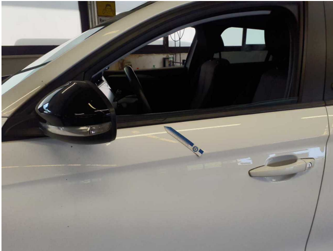
Damage 3: Door - front left side: Strip - outer - Scratch(es) - Replace
