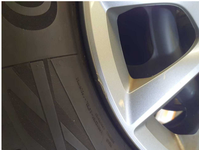
Damage 1: Wheel / tyres: Wheel cover - rear left side (+verformt) - Scratch(es) - Replace
